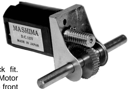
Take chosen motor gearbox combination and check fit. Shown are Connoisseur items, a Universal Floating Motor Mount with a 40:1 gear set and a 1833 motor driving the front axle. This is a straight fit between the front axle bearings with no adjustment for side play needed.
