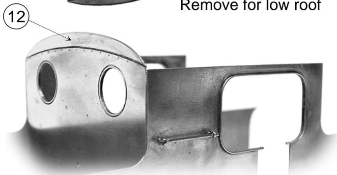
Ensure a snug fit between the cab sides & solder cab front to the slot in the footplate & flush with the front edge of cab.
