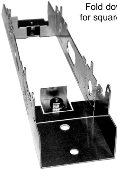
Fold down the chassis sides to 90 degrees check for square. Reinforce with solder along fold.
