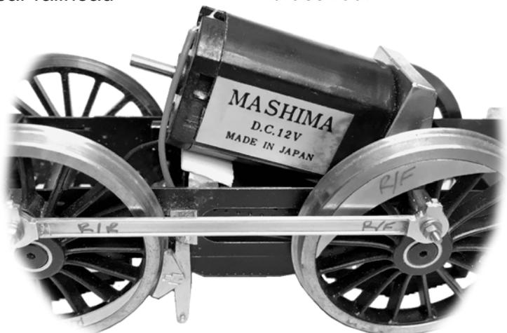
Although the prototype has rigid chassis frames with radial axles for the leading and trailing wheels this kit is a departure in that it includes a bogie at either end. This is to enable the locomotive to traverse curves and incorporate the close fitting wheel guards that are a distinctive feature of the F3.
