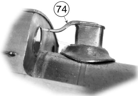
If using the early encased safety valve bonnet one will need the etched levers 74 soldered together.
